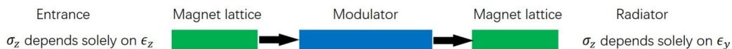
Fig. 5 (Color online) Schematic layout of applying TLC dynamics for bunch compression. (Figure adapted from Ref. [33])
