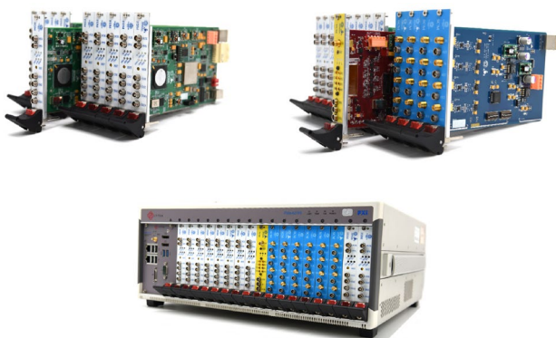
Fig. 5 (Color online) Photography of electronics modules (top left: FDM, top right: TCM and signal conditioning modules, bottom: read-out crate)
