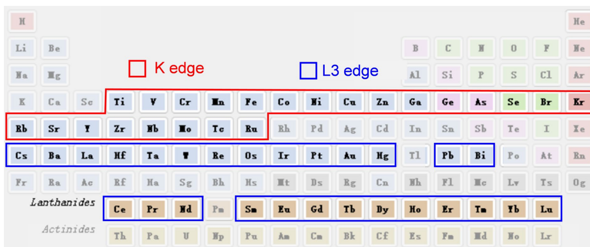
Fig. 11 (Color online) Elements measured on a BL17B XAFS experimental platform
