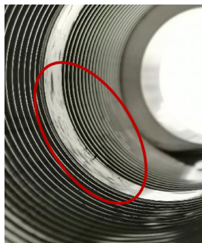
Fig. 20 (Color online) Contaminants inside the bellows
