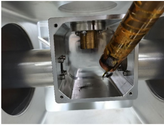
Fig. 10 (Color online) Coupler with a burnt inner conductor
