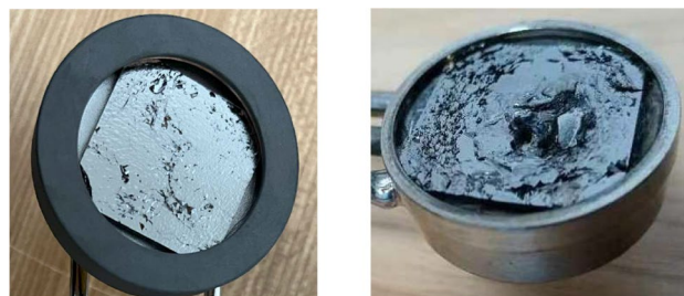
Fig. 5 (Color online) Picture of HOPG target before (left) and after 1.34 \times 10^7 \mu\text{C} beam dose bombardment (right)
