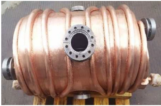
Fig. 9 (Color online) Finished HWR030 Nb-Cu composite cavity
