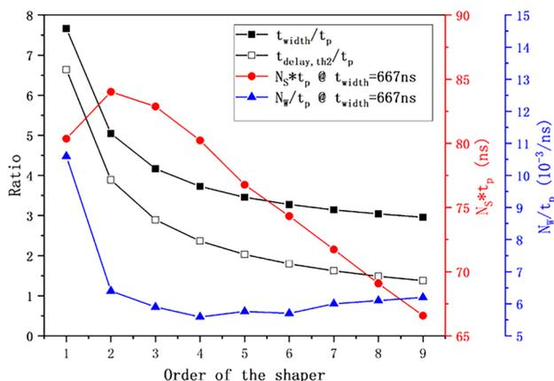
**Fig. 6** (Color online) Ratio of output-signal width  $t_{\text{width}}$  to peak time  $t_p$  and ratio of input-signal interval  $t_{\text{delay}}$  to peak time  $t_p$  for different filter orders
