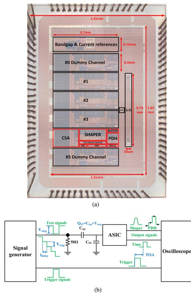
**Fig. 9** (Color online) (a) Microphotograph of the SECALROC3 ASIC. (b) Structure of the setup for chip measurement
