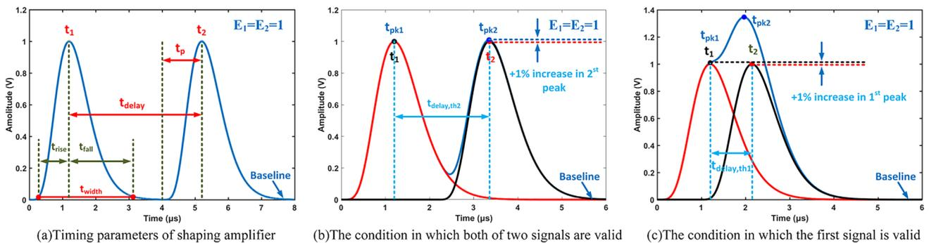
**Fig. 5** (Color online) Shaping-amplifier output-signal waveforms and associated time parameters
