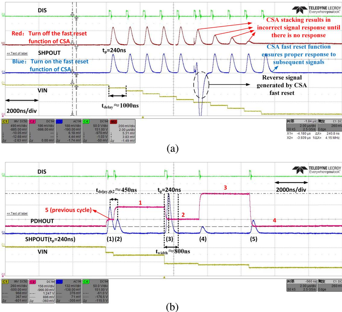
**Fig. 10** (Color online) (a) CSA fast-reset function test results. (b) Shaper and PDH-circuit test results with output piled-up signal
