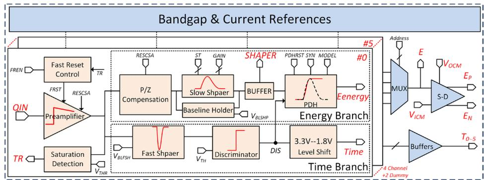
and level shifter. The fast shaper is used to decrease the signal width and increase the count rate of the time channel [23, 24]. A hysteresis comparator is used to generate a pulse signal, and the output pulse leading-edge indicates the TOA. The level shifter can shift the 3.3 V pulse signal to 1.8 V to match the power supply of the time-to-digital converter [12].
