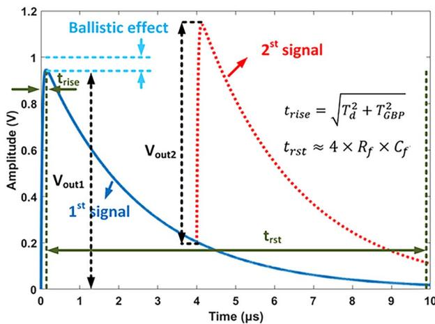
**Fig. 3** (Color online) Charge-sensitive amplifier output-signal waveforms and associated time parameters
