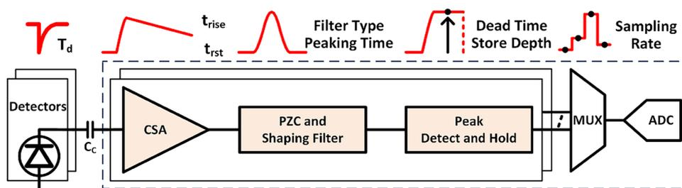
**Fig. 2** (Color online) Block diagram illustrating the ASIC architecture
