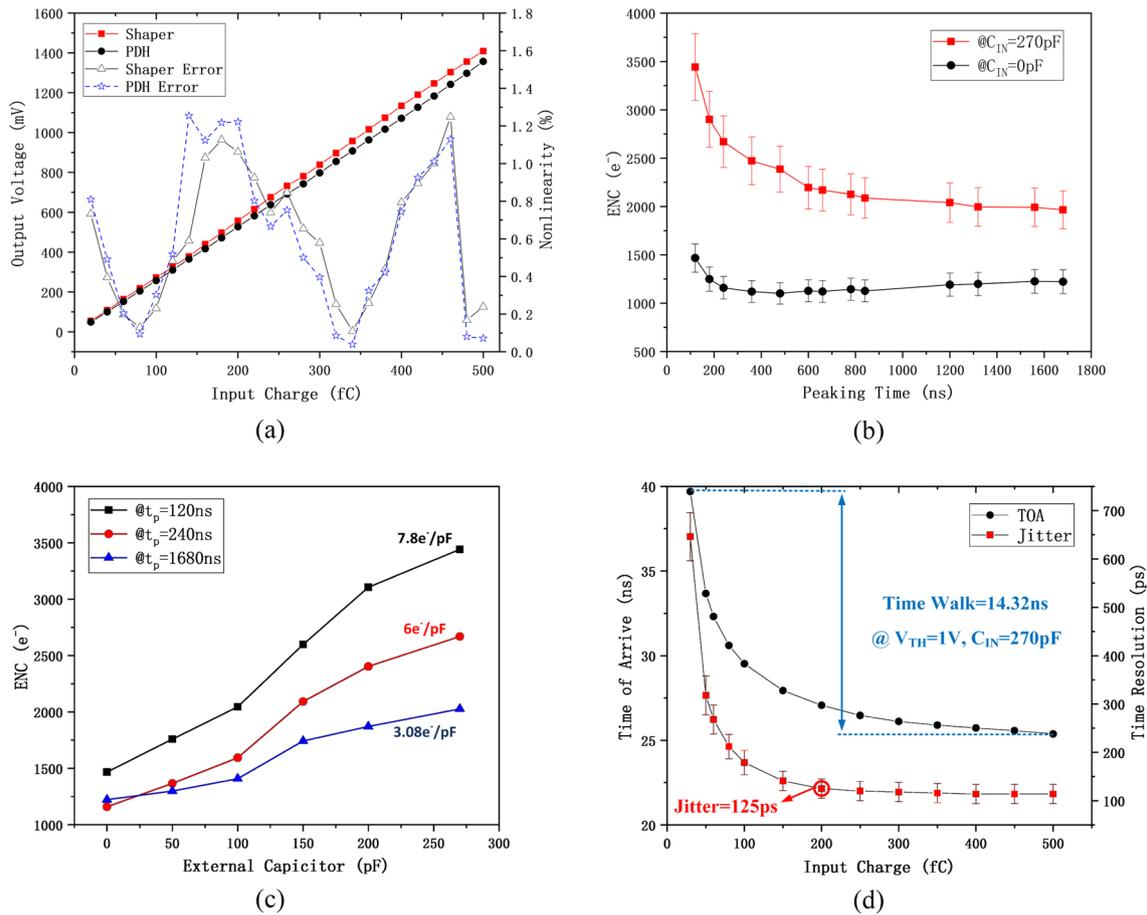
**Fig. 11** (Color online) (a) Linearity error measured at a 600 ns peak time. (b) Measured ENC versus peak time at room temperature. (c) Measured ENC versus external capacitance. (d) Measured TOA and time resolution versus input charge with a threshold of 20 fC
