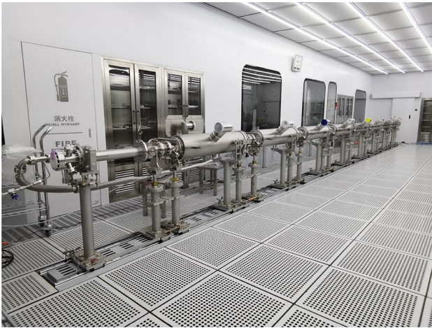
Fig. 2 (Color online) Cavity-string assembly in class 10 cleanroom
