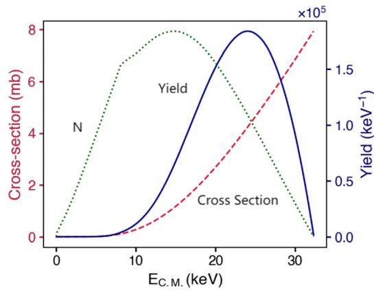
**Fig. 22** Neutron yield contributed by deuterium ions with different  $E_{c.m.}$  energies. Three data lines are shown in this chart: the number of the ions from the experimental diagnostic (dotted green line),  $D(d,n)^3\text{He}$  cross section (dashed red line), and calculated neutron yield (solid blue line) [199]
