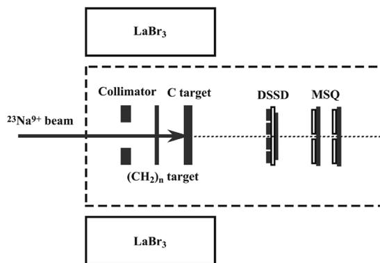
**Fig. 18** Setup of the  $^{23}\text{Na}+p$  thick-target experiment [114]
