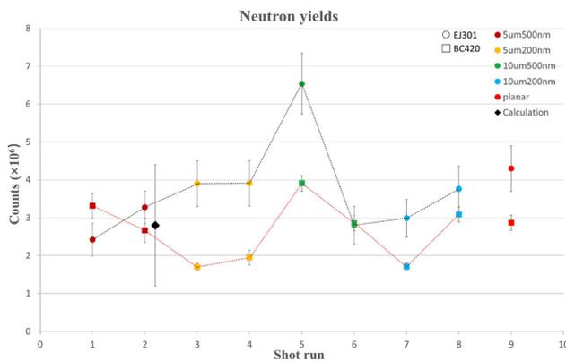
**Fig. 23** (Color online) Neutron yields with statistical uncertainties from EJ301 and BC420 detection and different target parameters. The circles represent the results of EJ301 detection and the squares represent those of BC420. The black diamond represents the results of the numerical calculation with the optical diagnostics approach for the 2nd shot run. Different colors correspond to different target parameters [199]
