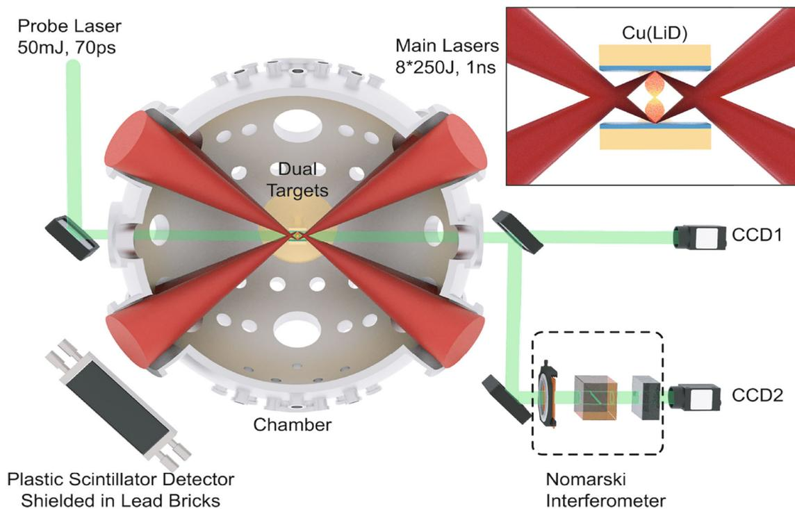
**Fig. 21** (Color online) Schematic layout of the experimental setup. The materials of the main targets are lithium deuteride (LiD) with density  $\rho_{\text{LiD}} = 0.906 \text{ g/cm}^3$  (see the enlarged illustration in the upper right corner). The counter-streaming plasmas are produced from the
