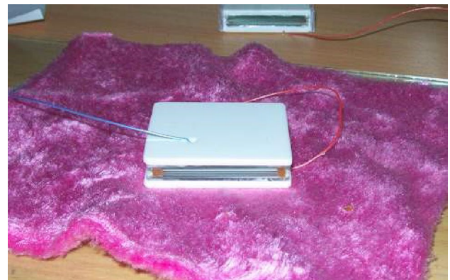
Fig. 1 (Color online) First MRPC prototype produced by USTC, with an active area of 4\text{ cm} \times 4\text{ cm} and single-channel readout
