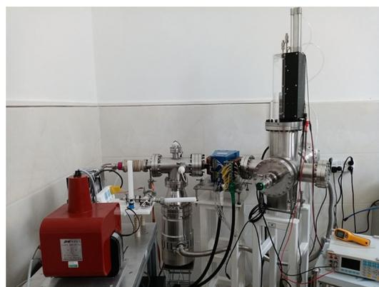
**Fig. 6** Photograph of the 50 kV ECR ion source platform. (Color figure online)
