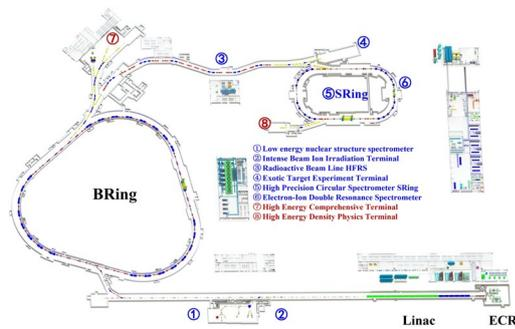
**Fig. 1** (Color online) Layout of the accelerator complex of HIAF
