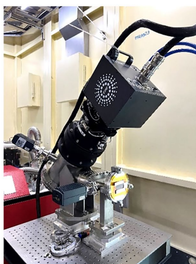
Fig. 10 (Color online) Photograph (left) and sequence of Ag foil K -edge EXAFS (right) acquired using FReLoN 2D detector at D -Line
