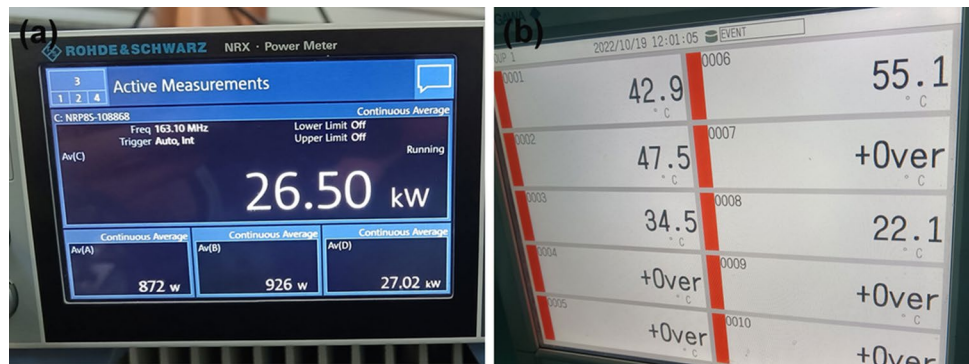
Fig. 9 (Color online) Conditioning result: a power; b temperature distribution
