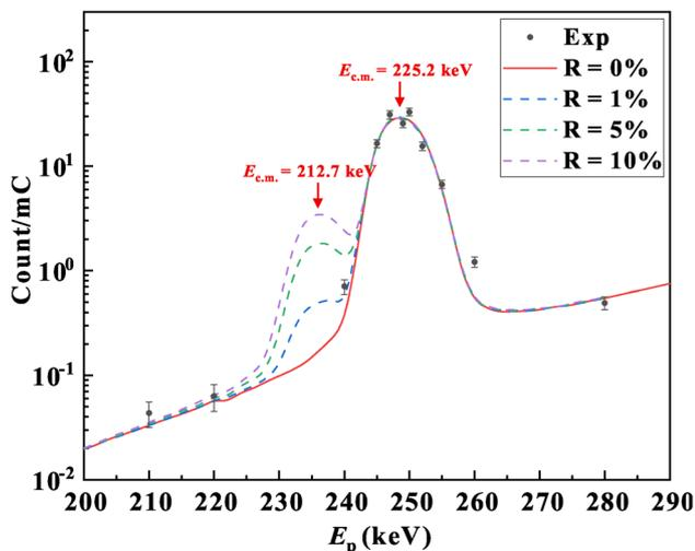
**Fig. 5** Geant4 simulated influence of the previously expected  $E_{\text{c.m.}} = 212.7$  keV resonance to the measured  $(p, \gamma)$  yields. The legend “ $R$ ” refers to the strength ratio of  $\omega\gamma_{(p, \gamma)}^{212.7} / \omega\gamma_{(p, \gamma)}^{225.2}$ , e.g.,  $R = 1\%$  denotes a 212.7-keV resonance strength assumed to be 1% that of the 225.2-keV resonance
