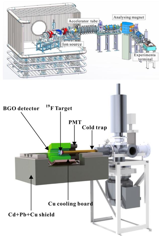
**Fig. 2** (Color online) 3D schematic of the JUNA platform (upper panel) and experimental setup (lower panel) [22]. In the lower panel, the proton beam came in from the right side, passed through a cold trap, and impinged on the fluorine target. The  $\gamma$ -rays emitted were detected by a near  $4\pi$  BGO detector array composed of eight identical segments. The BGO array was shielded by 5-mm Cu, 100-mm Pb, and 1-mm Cd layers from inside to outside [31]
