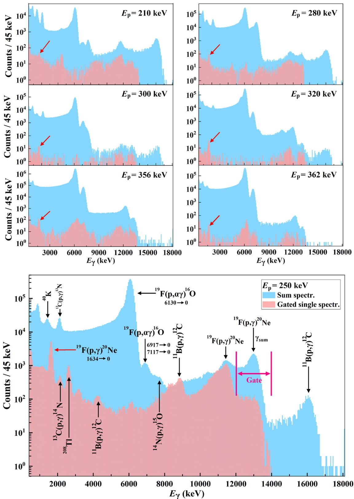
**Fig. 3** (Color online) (Upper panel) Sample  $\gamma$ -ray spectra taken at beam energies of  $E_p = 210$ – $362$  keV. The red arrows indicate the 1634-keV peak, which corresponds to the  $\gamma$  transition from the first excited state to the ground state in  $^{20}\text{Ne}$ . (Lower panel) Enlarged
