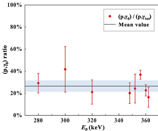
**Fig. 4** Yield ratio of the  $(p, \gamma_0)$  branch to the total one  $(p, \gamma_0) + (p, \gamma_1)$ . Here, the error bars shown represent only the statistical error; the black line and shadowed area represent the mean value (26.5%) and total error (5.2%), respectively
