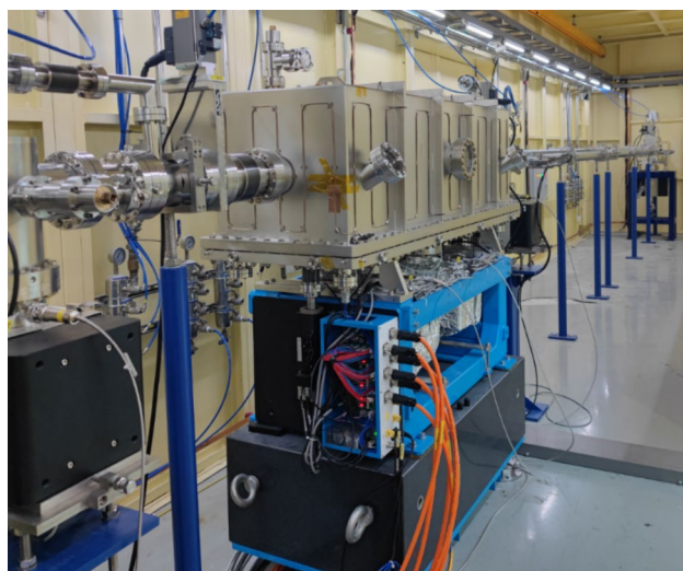
Fig. 4 (Color online) Toroid focusing mirror system equipped at BL11B
