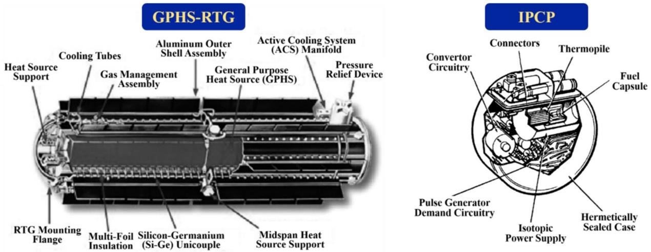
Fig. 1 Structures of GPHS-RTG and IPCP
