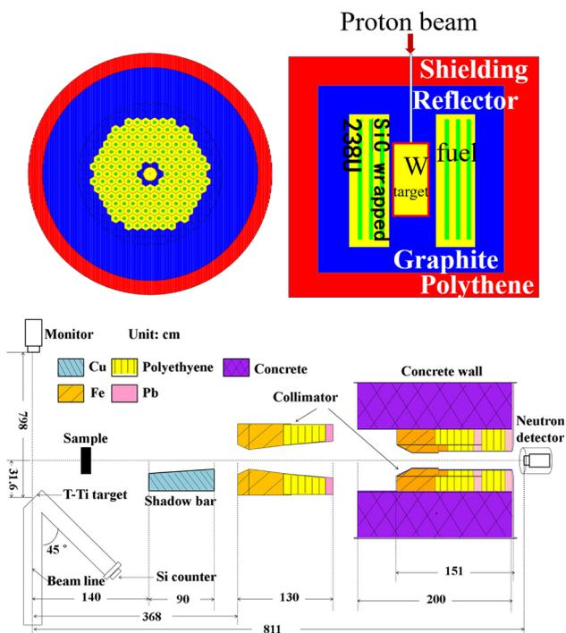
**Fig. 6** (Color online) Benchmarking of evaluated nuclear data for ADS with neutron nuclear data benchmark experiment setup at CIAE
