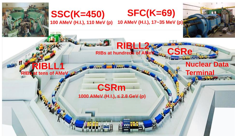
**Fig. 2** (Color online) Nuclear data measurement facility in the nuclear data terminal of HIRFL-CSR
