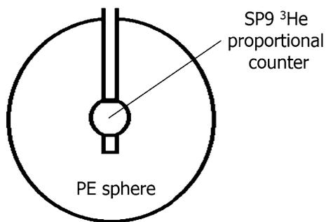
Fig. 1 Schematic of PS and SP9 <sup>3</sup>He proportional counter part
