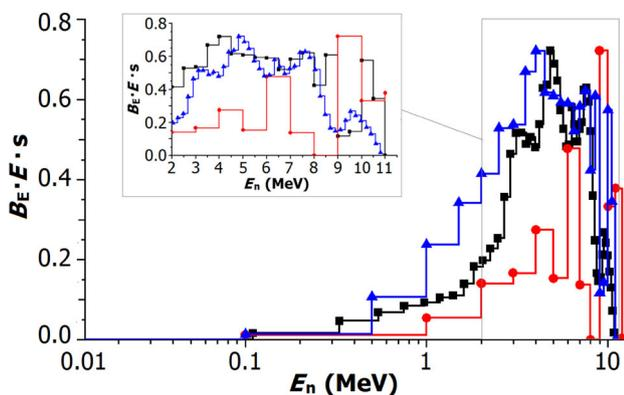
**Fig. 5** (Color online) Neutron source spectra of the  $^{241}\text{Am-Be}$  evaluated by ISO 8529-1 (filled square), and simulated with (filled triangle) and without (filled circle) 4 eV neutron process.  $B_E$  is the spectral source strength, and  $E_n$  is neutron energy
