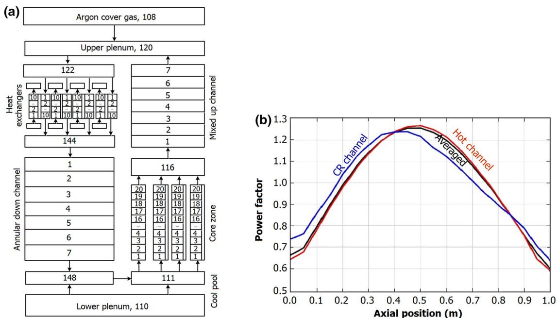
**Fig. 3** (Color online) Model of SNCLFR-100 primary cooling system **a** Nodalization of RELAP5 and **b** Axial power density distribution
