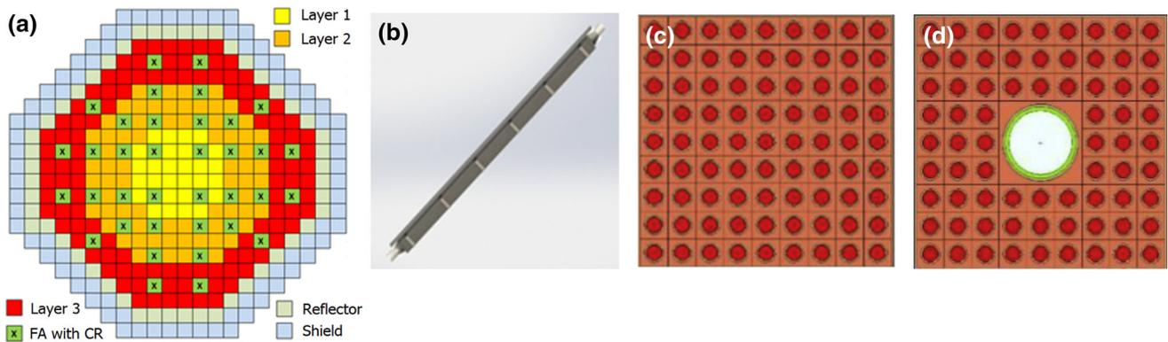
**Fig. 2** (Color online) Scheme of SNCLFR-100 core. **a** Core layout, **b** 3D drawing of the assembly, **c** Fuel assembly, **d** Control rod assembly
