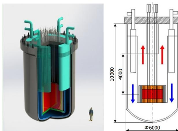
**Fig. 1** (Color online) Schematic diagram of SNCLFR-100 primary cooling system
