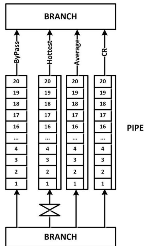
Fig. 4 Nodalization of the core zone for flow blockage
