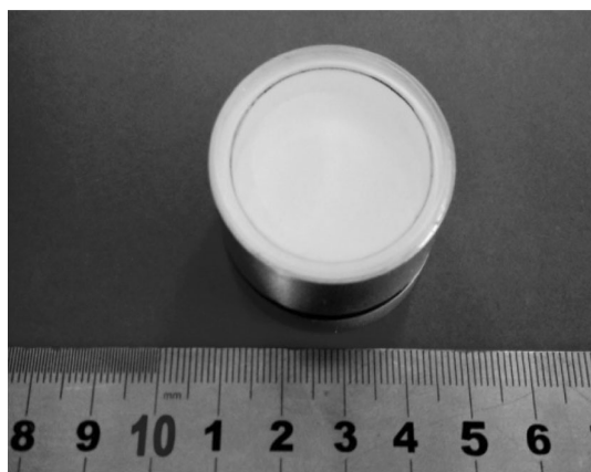
Fig. 1 Photograph of CLYC crystal 25.4 mm in diameter and 15 mm in thickness grown at BGRI. The crystal is packaged in an aluminum enclosure
