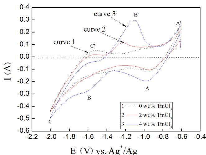
Fig. 1. (Color online) Cyclic voltammograms obtained at liquid Zn electrode ( $S = 1.08$  cm<sup>2</sup>) at 723 K in LiCl-KCl melt (curve 1); LiCl-KCl-TmCl<sub>3</sub> (2 wt.%) melt (curve 2); LiCl-KCl-TmCl<sub>3</sub> (4 wt.%) melt (curve 3); scan rate, 0.2 V/s.
