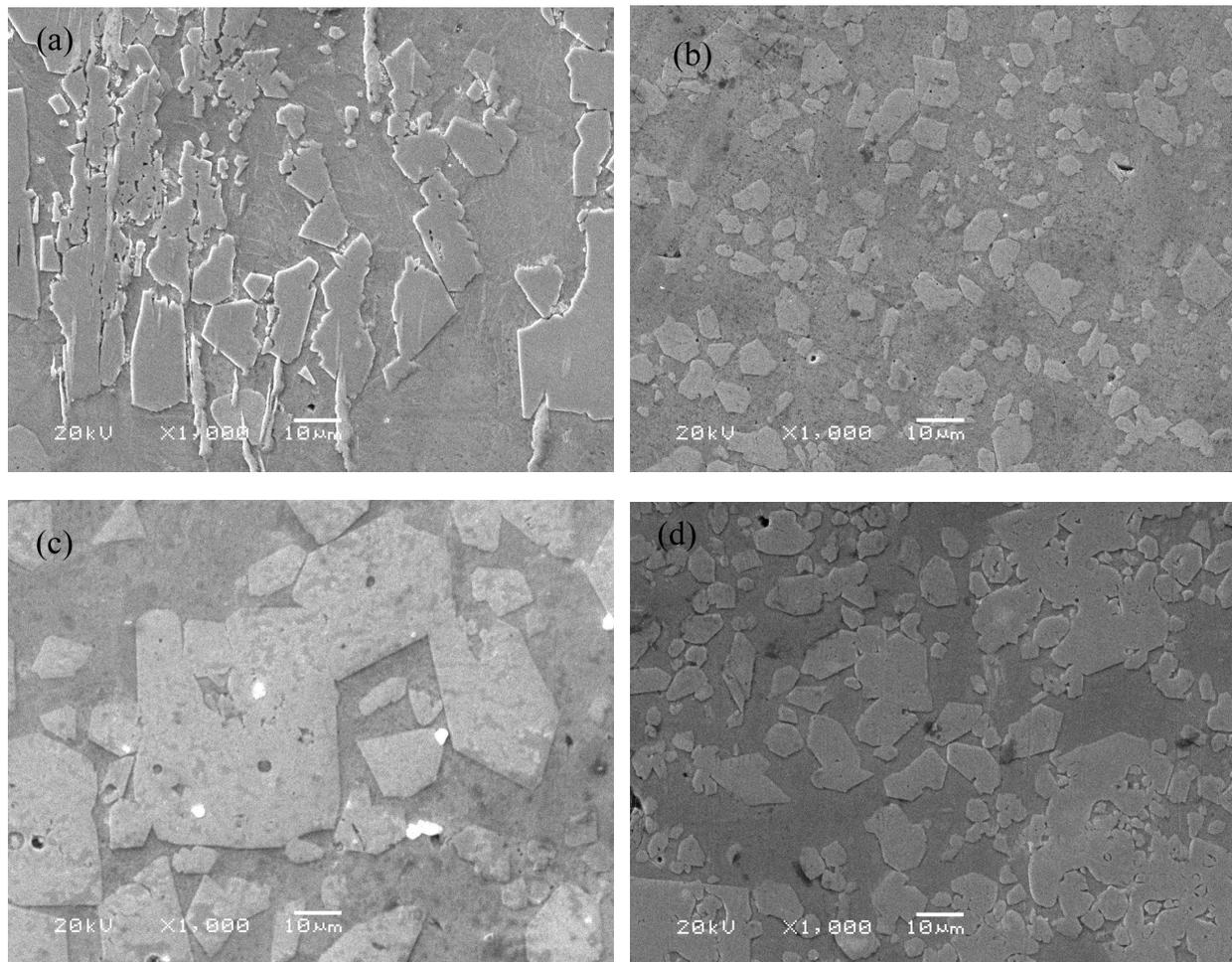
Fig. 5. Cross-sectional SEM (back scattering image) of Zn-Tm alloy obtained in LiCl-KCl-TmCl<sub>3</sub> (6 wt.%) melt at 723 K at liquid Zn electrode via galvanostatic electrolysis at (a) 200 mA/cm<sup>2</sup>, (b) 300 mA/cm<sup>2</sup> for 3 h, (c) 400 mA/cm<sup>2</sup> and (d) 500 mA/cm<sup>2</sup> for 2 h, respectively.
