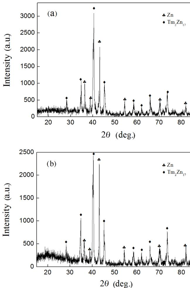
Fig. 4. XRD patterns of deposits obtained in LiCl-KCl-TmCl<sub>3</sub> (6 wt.%) melt at 723 K at liquid Zn electrode via galvanostatic electrolysis for 3 h at (a) 200 mA/cm<sup>2</sup>, (b) 300 mA/cm<sup>2</sup>, respectively.
