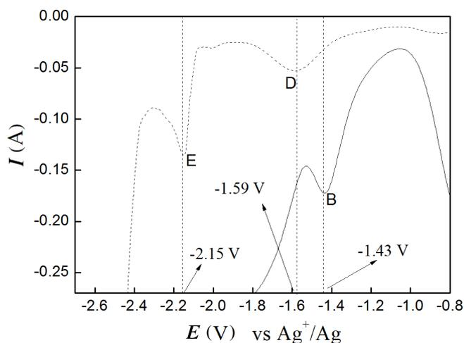
Fig. 2. Square wave voltammograms obtained in LiCl-KCl-TmCl<sub>3</sub> (2 wt.%) at a W electrode (dotted line) and liquid Zn electrode (solid line), respectively; pulse height, 25 mV; potential step, 1 mV; frequency, 15 Hz.
