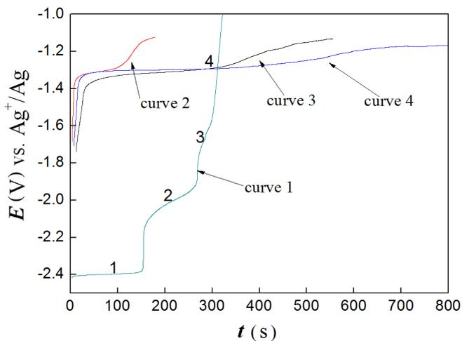
Fig. 3. (Color online) Open circuit chronopotentiometry curves obtained in LiCl-KCl-TmCl<sub>3</sub> (2 wt.%) melt at 723 K on a W electrode after potentiostatic electrolysis at  $-2.5$  V for 30 s (curve 1); at liquid Zn electrode after potentiostatic electrolysis at  $-2.5$  V for 2 s (curve 2), 5 s (curve 3) and 10 s (curve 4), respectively.
