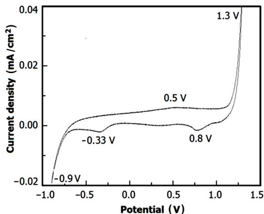
Fig. 2. Cyclic voltammogram of 1 mM KReO<sub>4</sub> in 1 M HCl at 298 K; Scan rate: 25 mV/s (Unit: Potential, V vs. Ag/AgCl).
