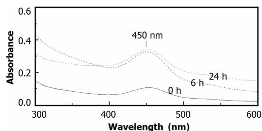
Fig. 6. Absorption spectra of electroreduced Re solution 0 h, 6 h and 24 h after electrolysis. Concentrations:  $[\text{HCl}] = 1 \text{ M}$ .
