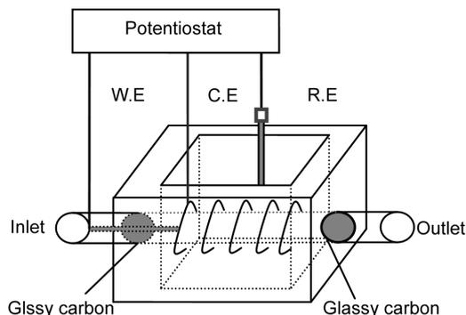
Fig. 1. The flow type high-efficient electrolysis cell.
