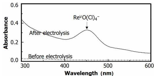
Fig. 4. Absorption spectra of Re solution before and after the electrolysis. Concentrations:  $[\text{HCl}] = 1 \text{ M}$ .
