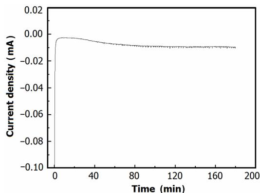
Fig. 3. Current in electrolysis of Re solution. [Re] = 1 mM; [HCl] = 1 M; flow rate: 0.8 cm<sup>3</sup>/min; Potential: -0.33 V (vs. Ag/AgCl).
