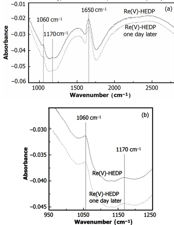
Fig. 8. ATR-IR spectra for Re(V)-HEDP complex at 298 K and pH 4 one day later. (a) wavenumber regions from 700  $\text{cm}^{-1}$  to 2800  $\text{cm}^{-1}$ , (b) from 950  $\text{cm}^{-1}$  to 1250  $\text{cm}^{-1}$ .
