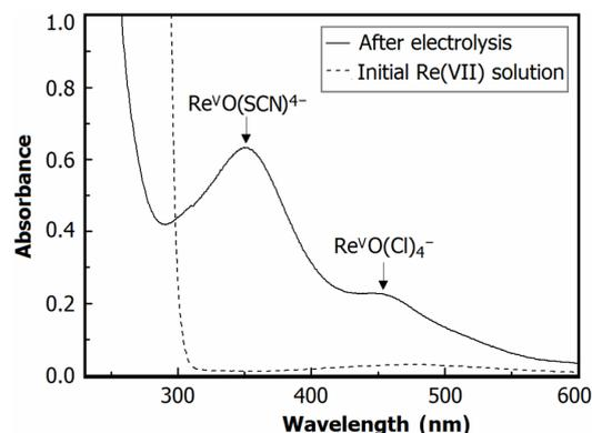
Fig. 5. Absorption spectra of Re solution modified with KSCN. Concentration:  $[\text{HCl}] = 1 \text{ M}$ ;  $[\text{KSCN}] = 0.1 \text{ M}$ .
