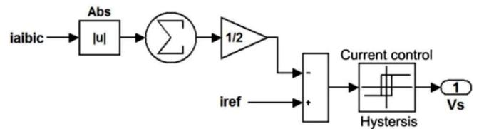
Fig. 5. Block diagram of hysteresis control scheme.
