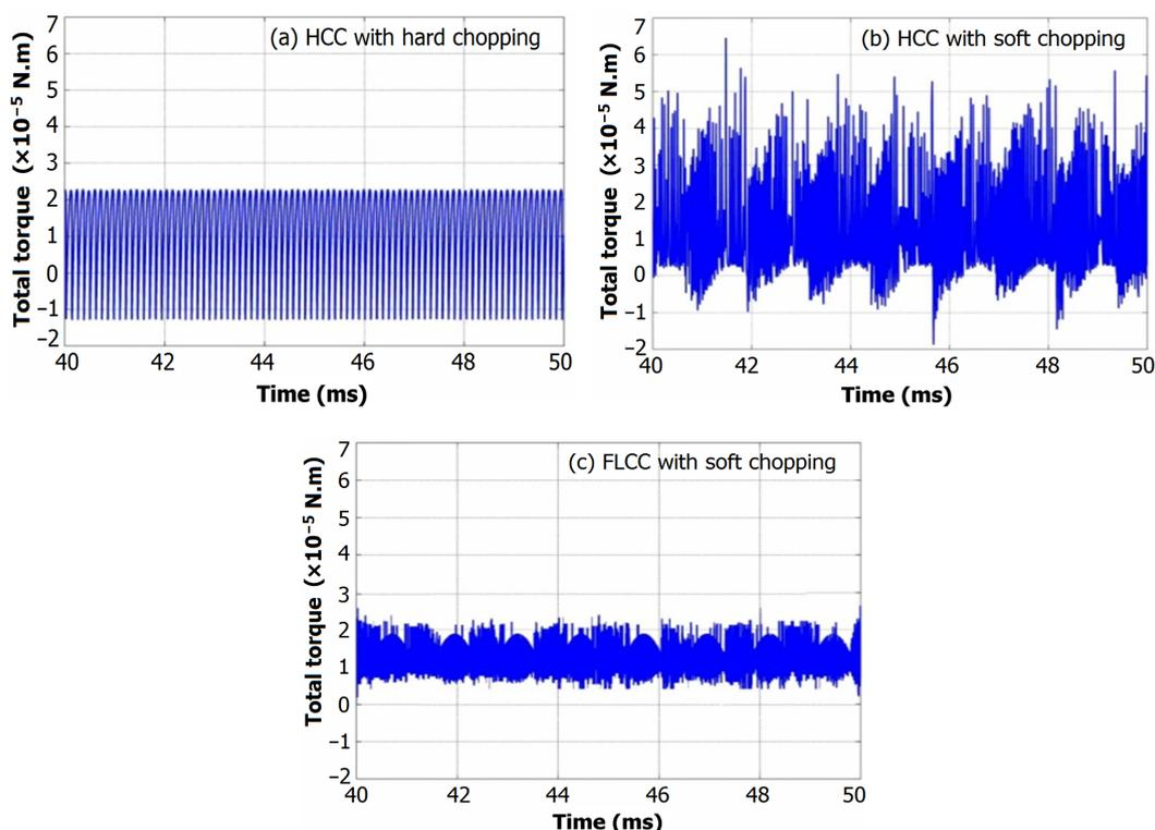
Fig. 9. (Color online) BLDC motor total torque in different chopping modes.
