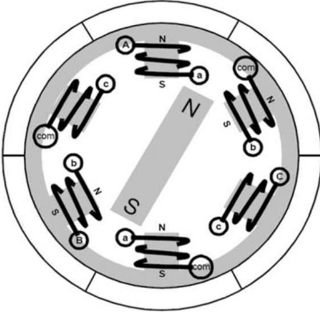
Fig. 1. Cross section of the three-phase BLDC motor construction.
