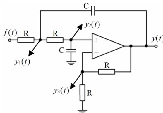
Fig. 1. Scheme of the Sallen-Key filter circuits.
