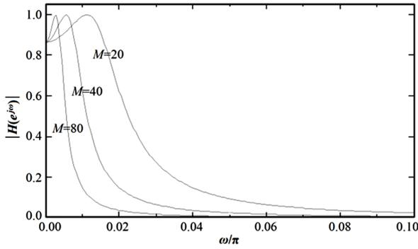
Fig. 3. The amplitude spectrum of  $H(e^{j\omega})$ .
