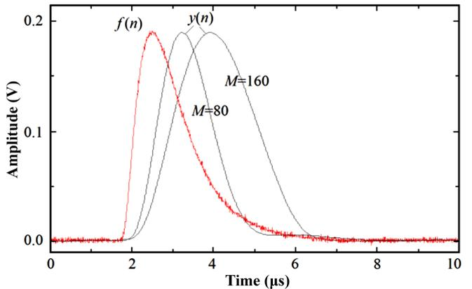
Fig. 6. (Color online) Response of the digital Gaussian shaping system with sampling signals from detecting a  $^{60}\text{Co}$  source.
