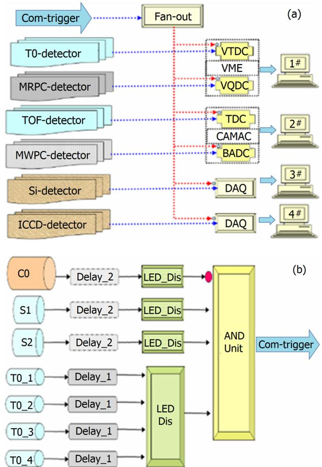
Fig. 2. (Color online) Data acquisition systems (a) and electronics trigger logic (b) in the beam test.
