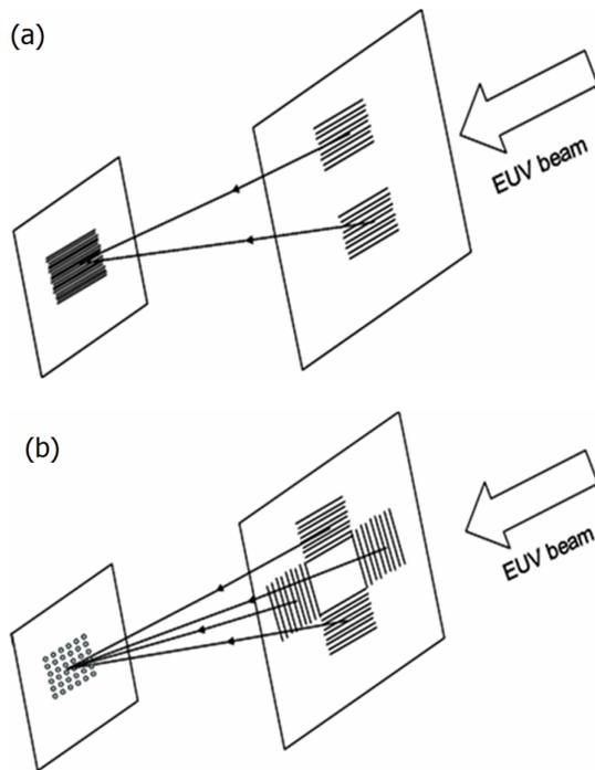
Fig. 2. (Color online) The schemes of grating based interference. 1D line patterns and 2D dot patterns will be fabricated respectively.
