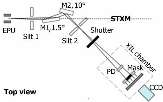
Fig. 1. (Color online) Schematic layout of the BL08U1B beamline.
