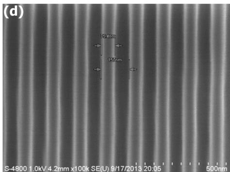
Fig. 5. (Color online) Fabrication process of the grating (a), SEM image of the two beam grating (b), and SEM image of the exposure result on PMMA (c), and on the user's MG resist (d).
