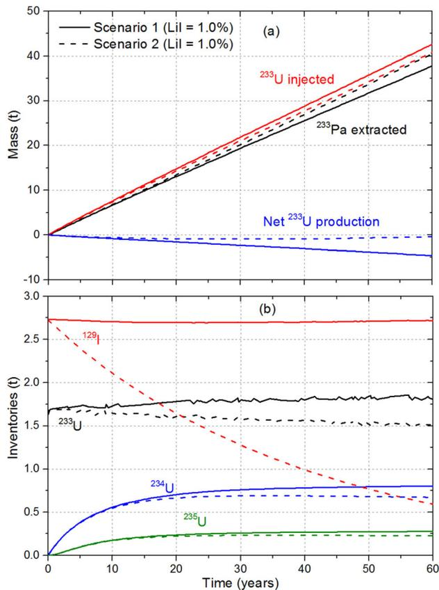
**Fig. 5** (Color online) **a** Net  $^{233}\text{U}$  production and **b** inventory of nuclides for both scenarios ( $\text{LiI} = 1.0\%$ ) during 60 years of operation
