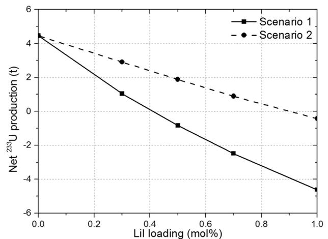
**Fig. 6** (Color online) Net  $^{233}\text{U}$  production at end of life as a function of initial loading of LiI for scenarios 1 and 2
