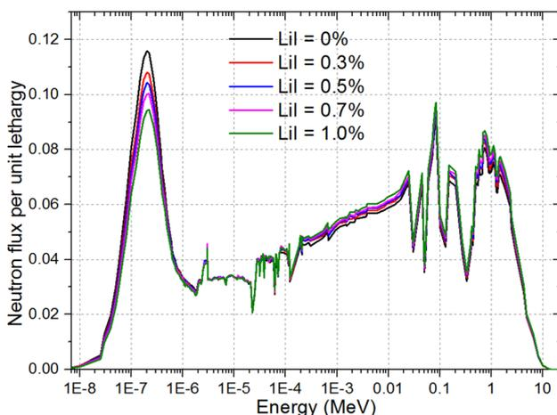
**Fig. 3** (Color online) Comparison of initial neutron spectra for different <sup>129</sup>I loadings
