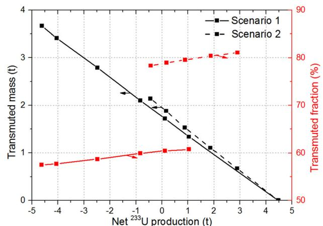
**Fig. 8** (Color online) Transmuted mass and fraction of  $^{129}\text{I}$  as a function of net  $^{233}\text{U}$  production for scenarios 1 and 2 at end of life
