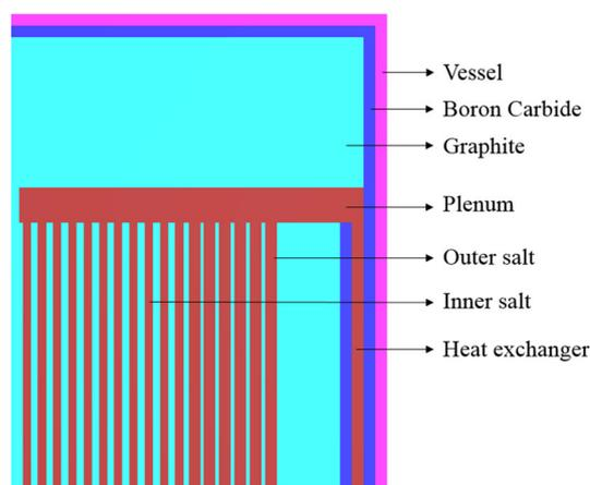
**Fig. 1** Cross section of SD-TMSR
