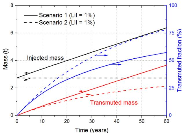
**Fig. 7** (Color online) Transmuted mass, injected mass, and transmuted fraction of  $^{129}\text{I}$  for scenarios 1 and 2 (LiI = 1.0%) during 60 years of operation
