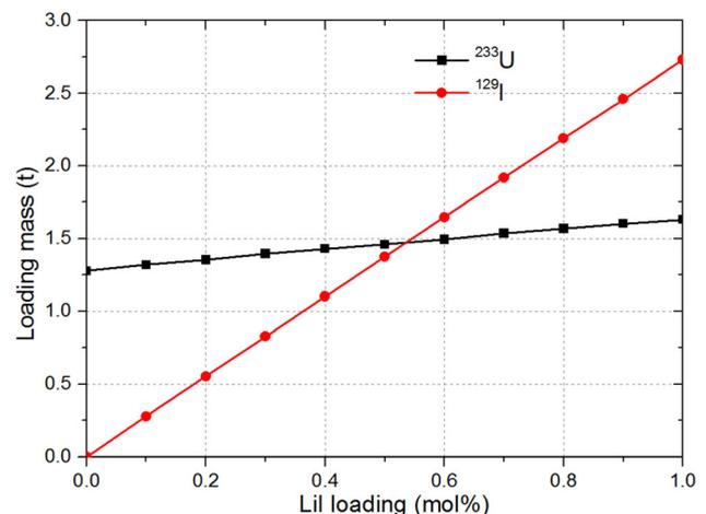
**Fig. 4** Initial <sup>233</sup>U and <sup>129</sup>I loadings as a function of <sup>129</sup>I molar proportion under critical condition
