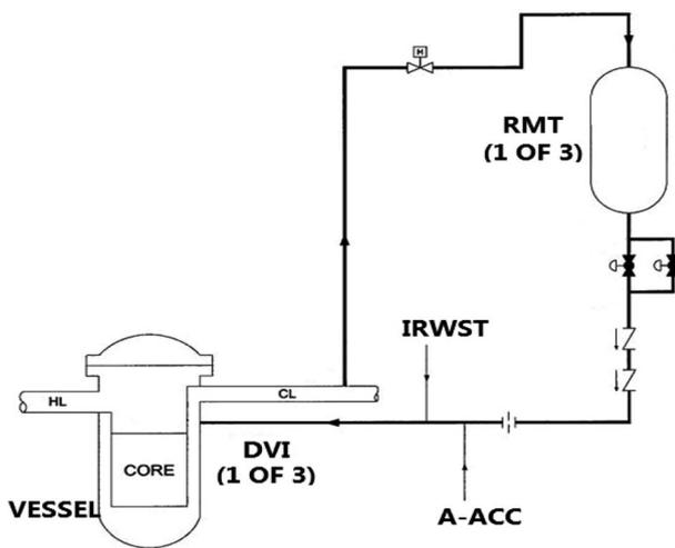
**Fig. 2** Schematic of RMT
