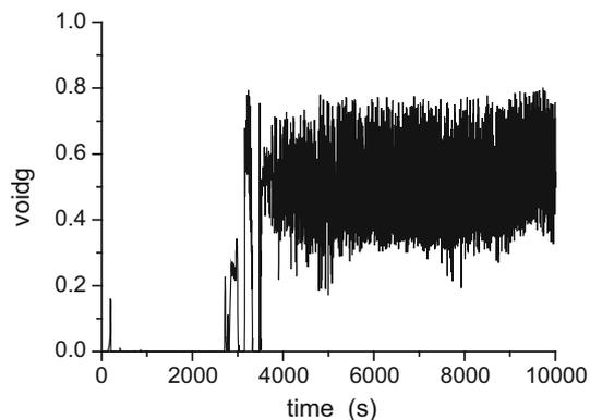
**Fig. 16** Void fraction of the core outlet zone
