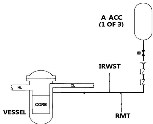
**Fig. 3** Schematic of A-ACC
