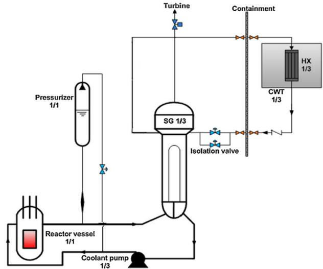
Fig. 6 Schematic of PEFS
