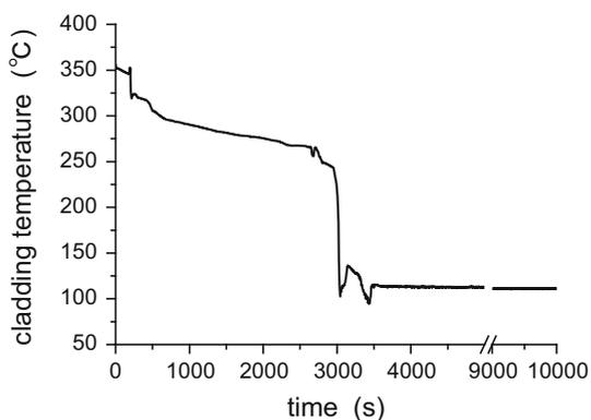
**Fig. 17** Maximum cladding temperature
