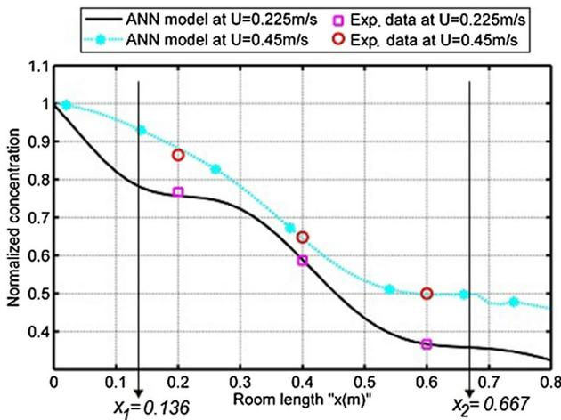
**Fig. 7** Axial distribution of normalized concentration at room height of  $y = 0.36$  m
