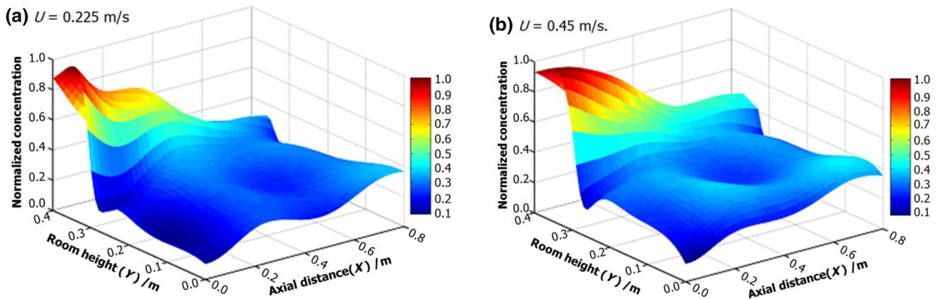
**Fig. 9** 3-D distribution of particle concentration in surface center at inlet velocity of **a**  $U = 0.225$  m/s and **b**  $U = 0.45$  m/s
