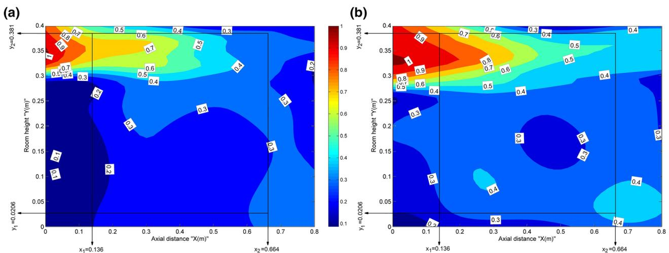
**Fig. 8** Simulation results for the distribution of particle concentration at the surface center. **a**  $U = 0.225$  m/s, **b**  $U = 0.45$  m/s
