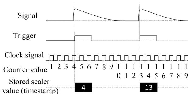
Fig. 6 The concept for recording the timestamps by the V830 module in a VME system
