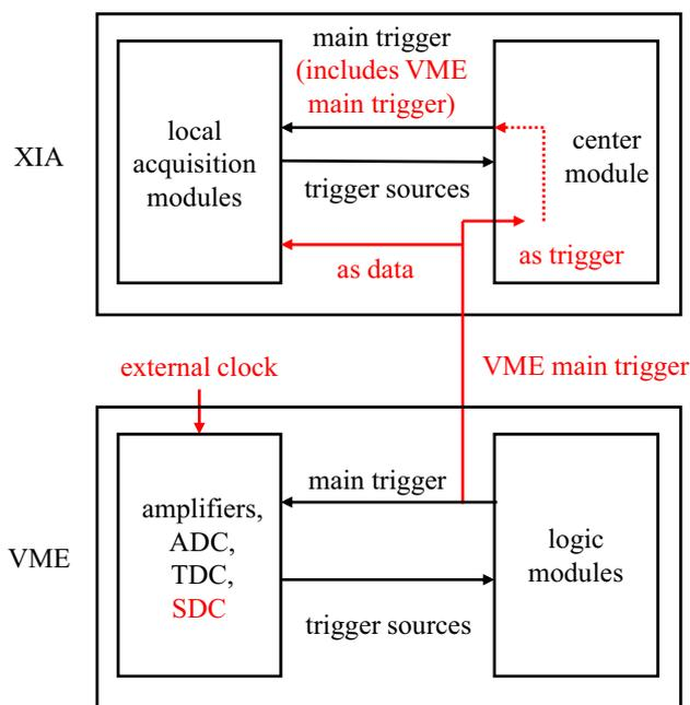
Fig. 5 Schematic of the combination between the XIA and the VME systems
