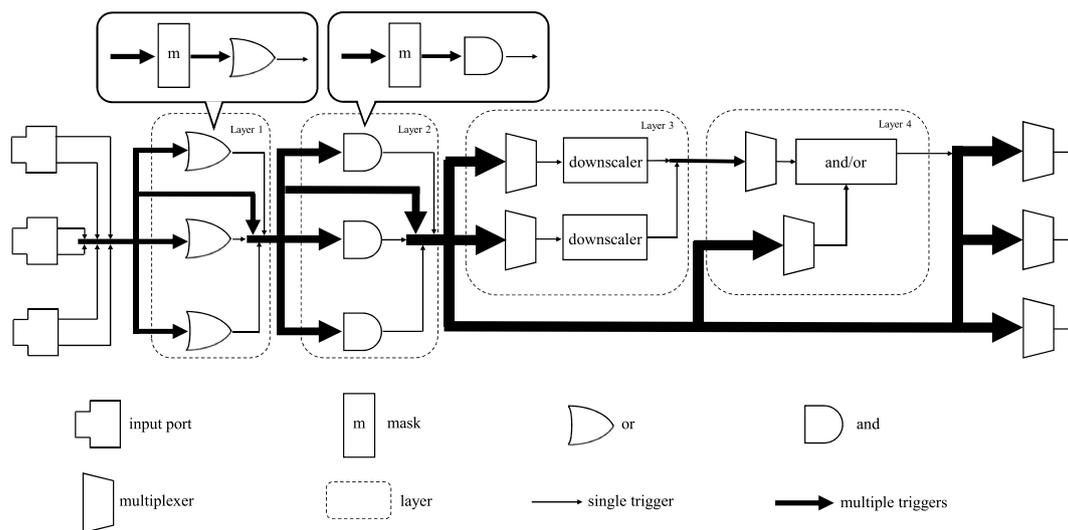
**Fig. 1** Schematic of the FPGA configuration with four layers as contained in the dashed line squares. The arrows show the digital signal flows with thickness proportional to the involved channel numbers.
