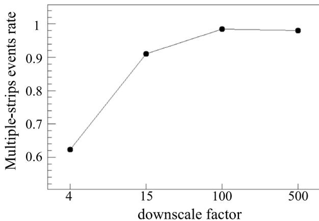
**Fig. 8** The multiple-strip event rate (in the zero-degree detector) normalized to the total event rate (filled circles), as a function of the downscaling factor
