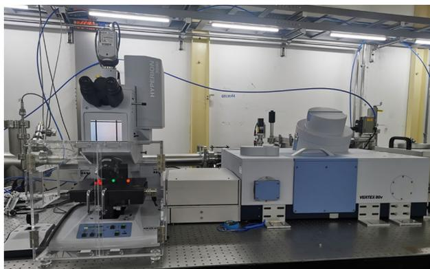
**Fig. 3** (Color online) IR spectrometer and microscope (VERTEX 80v and Hyperion 3000, Bruker)
