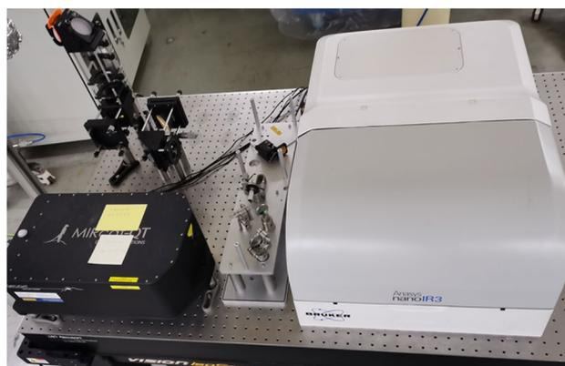
**Fig. 4** (Color online) Scan near-field optical microscope (NanoIR3, Bruker)
