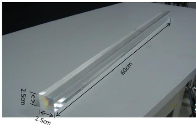
**Fig. 73** (Color online) The sample of BGO crystals
