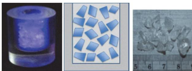
**Fig. 85** (Color online) Photograph of  $\emptyset 1'' \times 1''$  composite CLYC-Plastic detectors produced in RMD's (left), schematic of its structure (middle) and CLYC crystallites used in the composite detector. Reproduced from [364]
