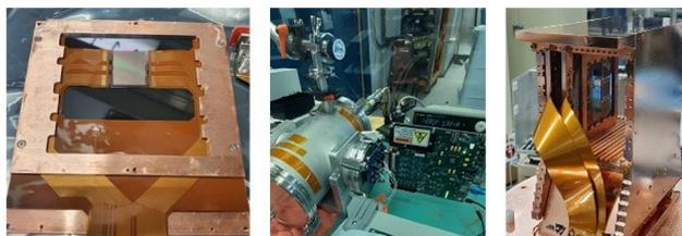
Fig. 1 (Color online) Left: Skipper-CCD in Cu module. Center and right: Setups at FNAL for testing packaged sensors. Reproduced from [9]
