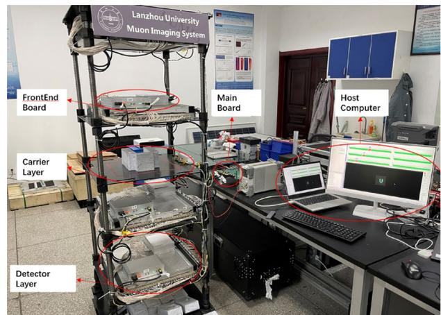
Fig. 78 (Color online) Lanzhou University Muon Imaging System, LUMIS. Reproduced from [351]
