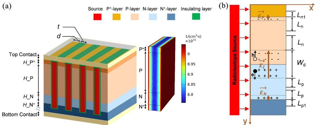
**Fig. 1** (Color online) **a** Schematic 3D diagram showing part of the proposed battery and the distribution of the electron–hole pair (EHP) generation rate in the innermost ridge with  $t = 0.8 \mu\text{m}$  and  $d = 1.2 \mu\text{m}$ ;
