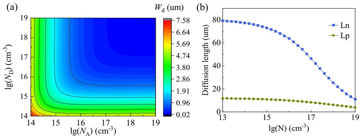
**Fig. 3** a Depletion region width and b minority diffusion length with doping concentration
