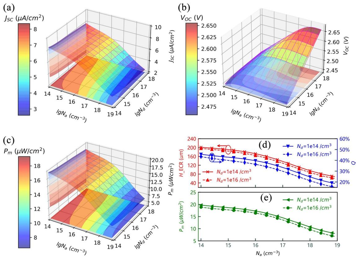
**Fig. 6** (Color online) Influence of  $N_a$  and  $N_d$  on **a**  $J_{sc}$ , **b**  $V_{oc}$ , and **c**  $P_m$ ; effect of  $N_a$  on **d**  $H_{ECR}$ ,  $Q$ , and **e**  $P_m$ .  $H_P=156 \mu m$ ,  $H_N=28 \mu m$ ,  $t=0.8 \mu m$ , and  $d=1.2 \mu m$
