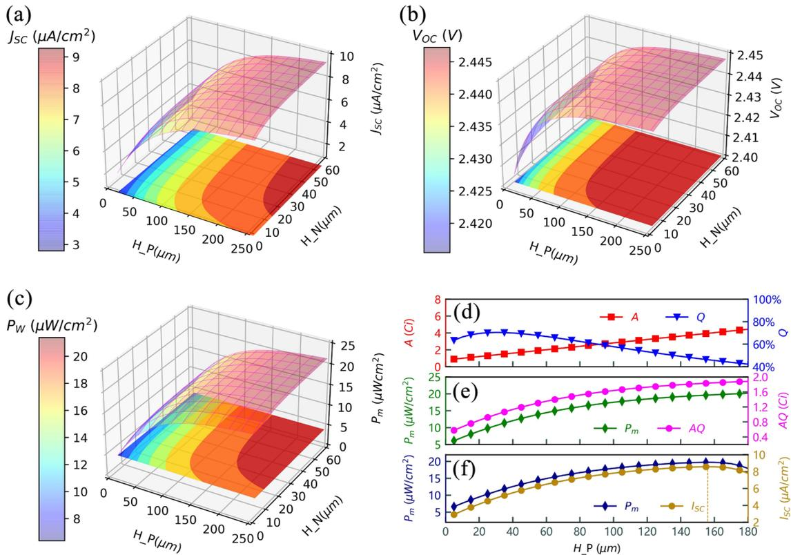
**Fig. 5** (Color online) Effects of  $H_P$  and  $H_N$  on **a**  $J_{SC}$ , **b**  $V_{OC}$ , and **c**  $P_m$  with varying  $H_{source}$ ; dependences of **d**  $A$ ,  $Q$ , **e**  $P_m$ , and  $A \cdot Q$  on  $H_P$  with  $H_N$  fixed at  $24 \mu\text{m}$ ; **f** dependence of  $P_m$  on  $H_P$  with  $H_{source}=200 \mu\text{m}$ .  $N_a$  and  $N_d$  are both set to  $1 \times 10^{14} \text{ cm}^{-3}$ ,  $t=0.8 \mu\text{m}$ , and  $d=1.2 \mu\text{m}$
