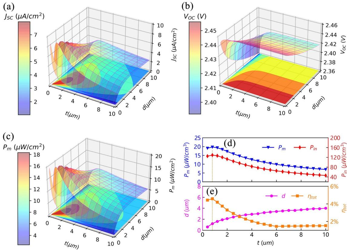
**Fig. 4** (Color online) Effects of the ridge spacing [ $t$ ] and ridge width [ $d$ ] on the **a**  $J_{SC}$ , **b**  $V_{OC}$ , **c**  $P_m$ ; the dependences of **d**  $P_m$ ,  $P_{in}$ , **e**  $d$ , and  $\eta_{tot}$  on  $t$ .  $N_a$  and  $N_d$  are both set to  $1 \times 10^{14} \text{ cm}^{-3}$ ;  $H_P$  and  $H_N$
