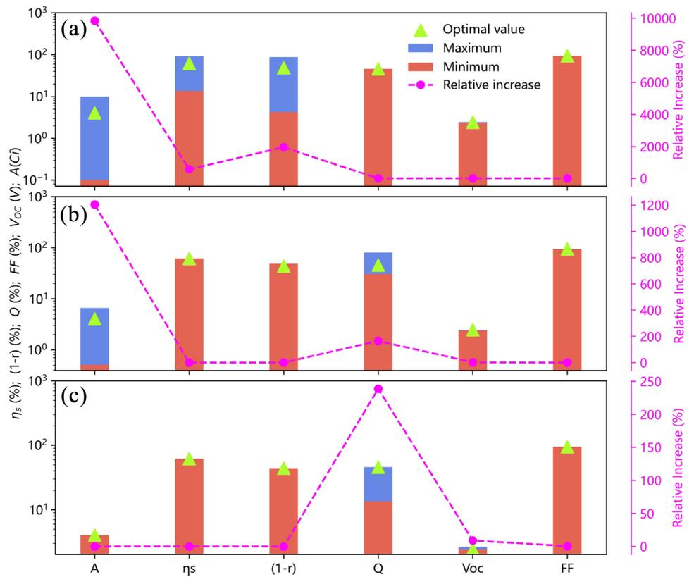
**Table 3** Comparison between our battery model results and previous works; optimization suggestions for the batteries in references; comparative analysis between the P<sup>+</sup>PNN<sup>+</sup> structure and the PN structure
