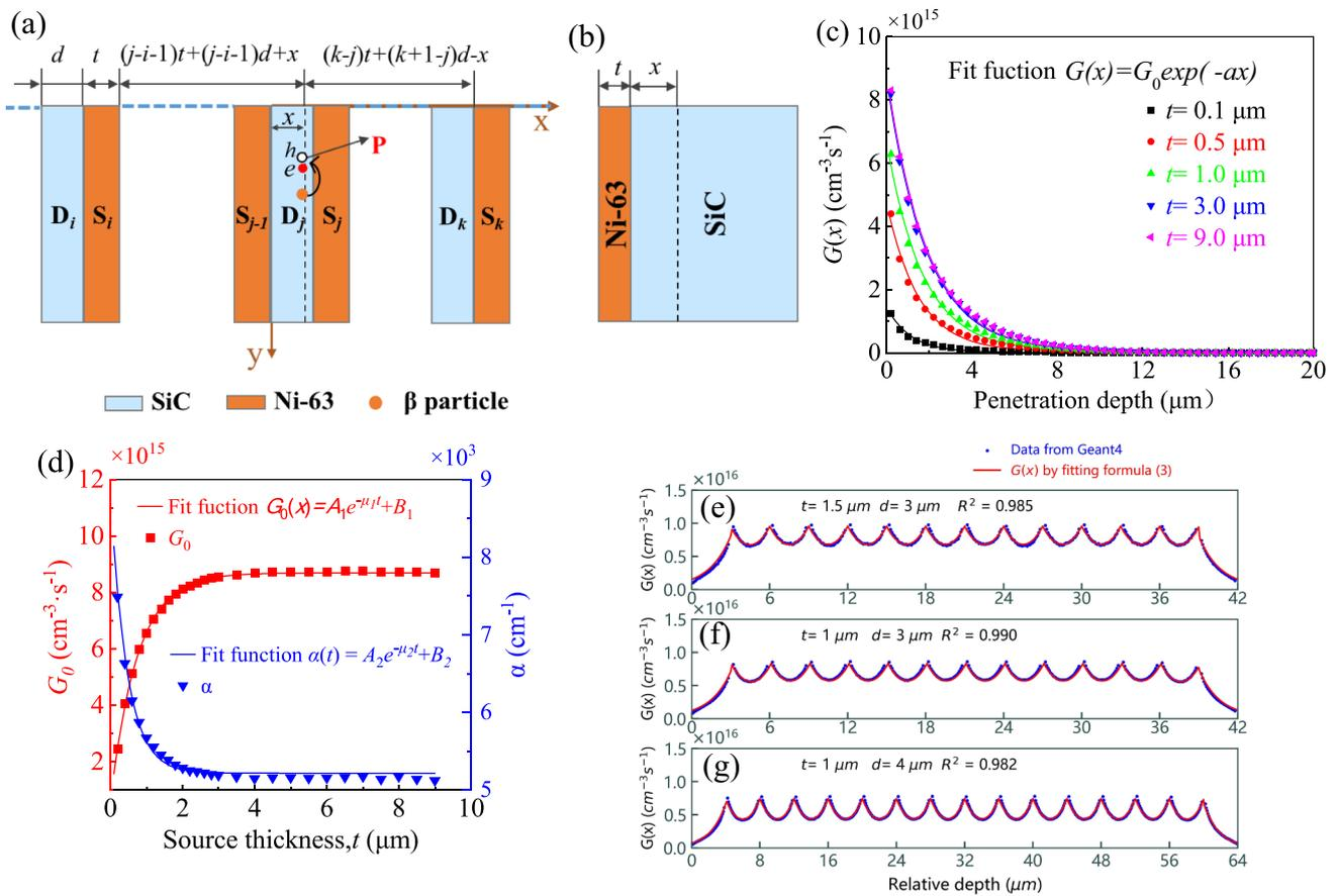
**Fig. 2** (Color online) Schematics of **a** 3D and **b** 2D converters; **c** EHP generation rates along penetration depth and **d** surface EHP generation rate and absorption coefficient for different source thicknesses in
