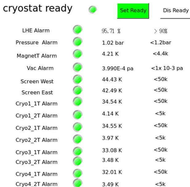
**Fig. 5** Desired and actual current values of the key parameters of cryogenic system
