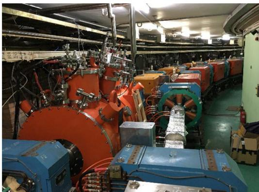
**Fig. 1** (Color online) 2.6-T 32-pole superconducting wiggler (SCW) for high-energy photon source test facility
