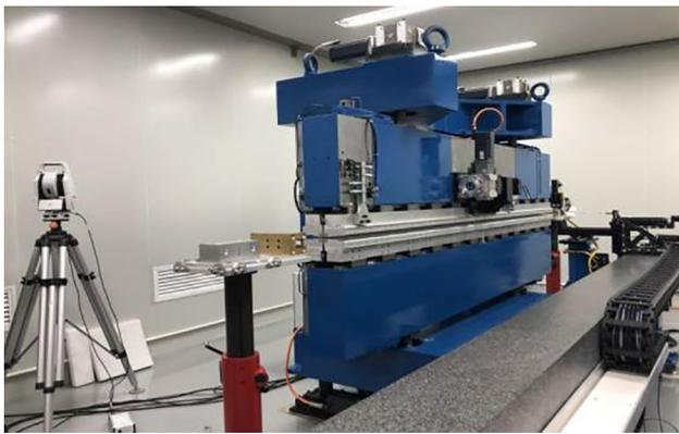
**Fig. 39** (Color online) Undulator magnetic fiducialization using magnetic landmark
