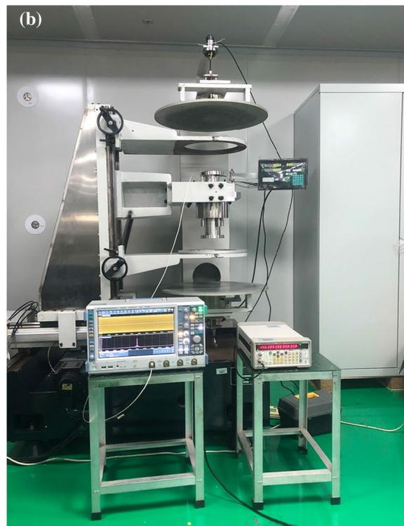
**Fig. 9** (Color online) Layout of the off-line test platform. On the left is a schematic of the stretched wire method, and on the right is a photograph of the beam analog measurement
