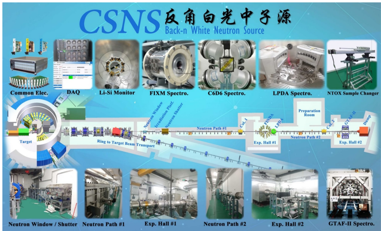
Fig. 1 (Color online) Back-n white neutron beam line and spectrometers for nuclear data measurements
