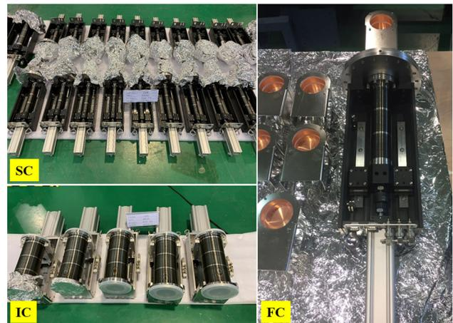
**Fig. 14** (Color online) SC, FC and thick IC of HUST-PTF. All detectors are driven by pneumatic actuators
