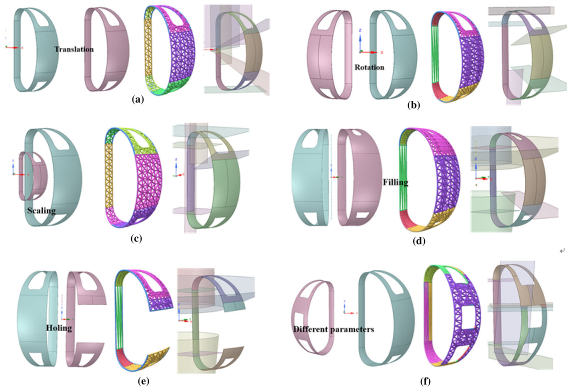
Fig. 16 (Color online) Robustness test of the intelligent segmentation algorithms. a Translation. b Rotation. c Scaling. d Filling. e Holing. f With a similar structure but with different parameters
