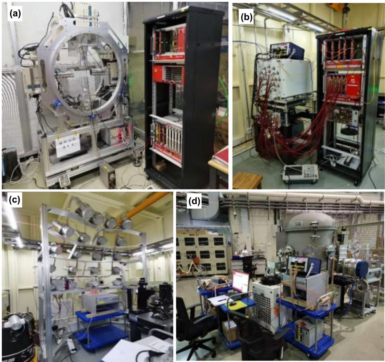
Fig. 12 (Color online) Four types of experimental spectrometers available in the SLEGS experimental station: gamma nuclear resonance fluorescence spectrometer (a), neutron flat-efficiency
