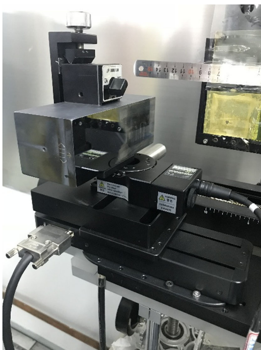
Fig. 3 (Color online) X-ray quasi-monochromator for X-ray pinhole camera at SSRF
