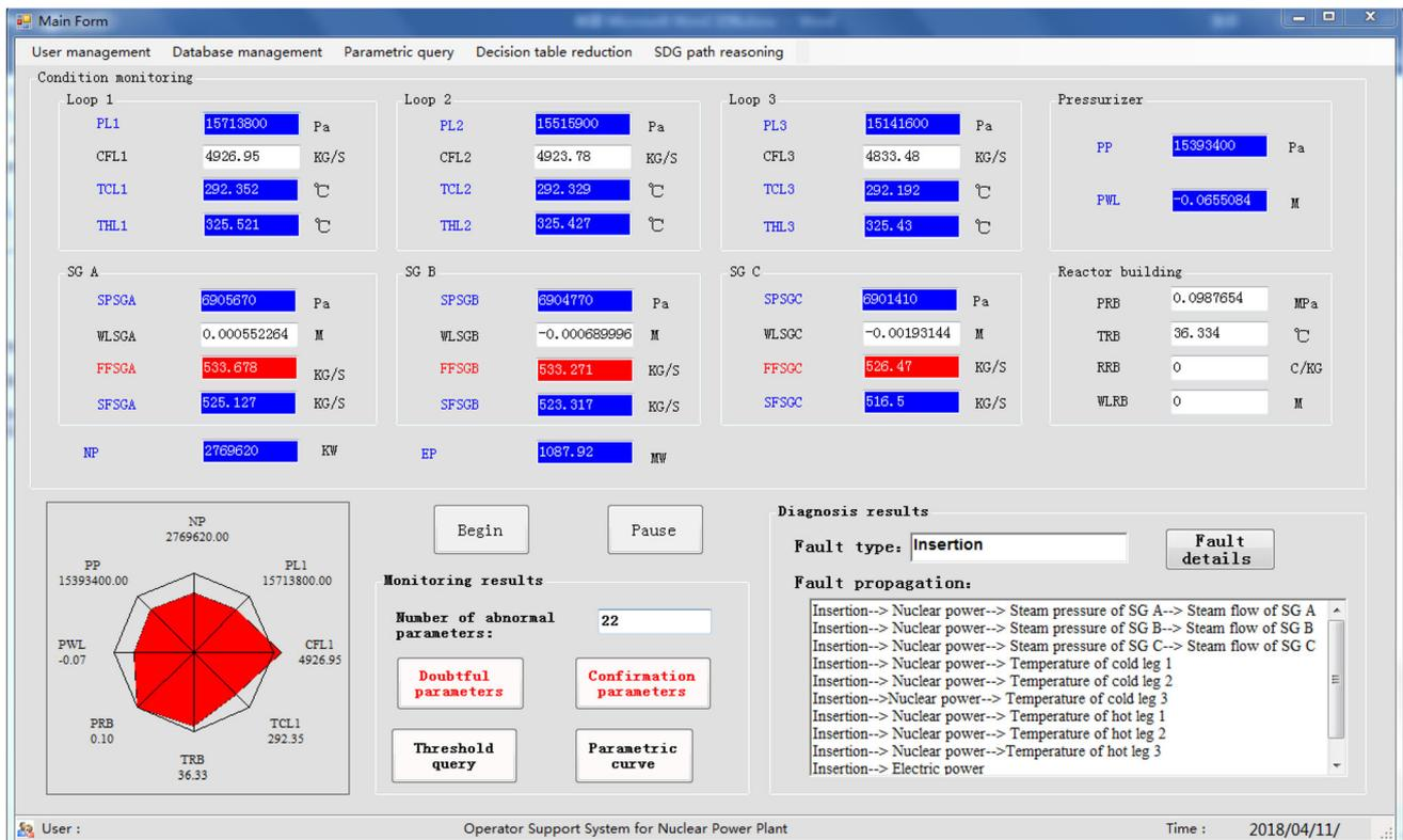
Fig. 9 Result of state monitoring and fault diagnosis for control rod insertion
