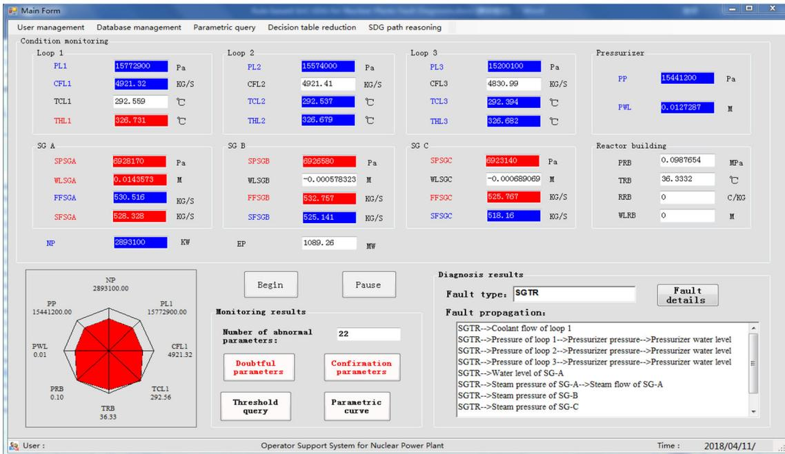
Fig. 7 Results of state monitoring and fault diagnosis of SGTR
