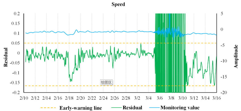
Fig. 8 Fault early warning effect of rotating speed signal (Color online)
