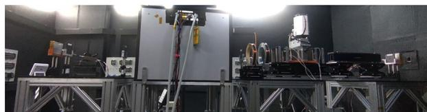
**Fig. 8** (Color online) Photograph of the experiment setup, corresponding to the schematic diagram in Fig. 6. A neutron beam with a diameter of 10 mm was produced using neutron slits. The distance from the detector to the neutron source was 14.99 m
