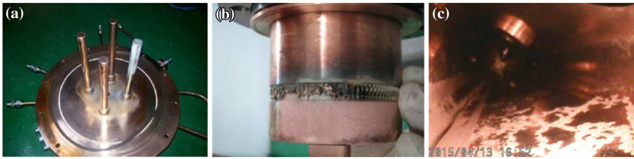
Fig. 12 Damage in RFQ-1 commissioning: a entrance plate with damaged rods, b coupler #4 with a burned RF contact spring, and c inner-surface damage status of RFQ-1
