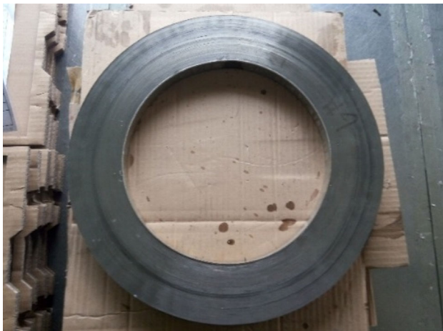
Fig. 2 (Color online) Large-sized MA core made of 1K107
