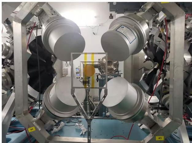
**Fig. 3** (Color online) Photograph of the  $C_6D_6$  detector system in the Back-n facility of the CSNS. A gold sample is placed in the aluminum sample holder
