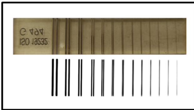
Fig. 10 Dual-line image quality indicator imaging based on in-lab DR imaging system
