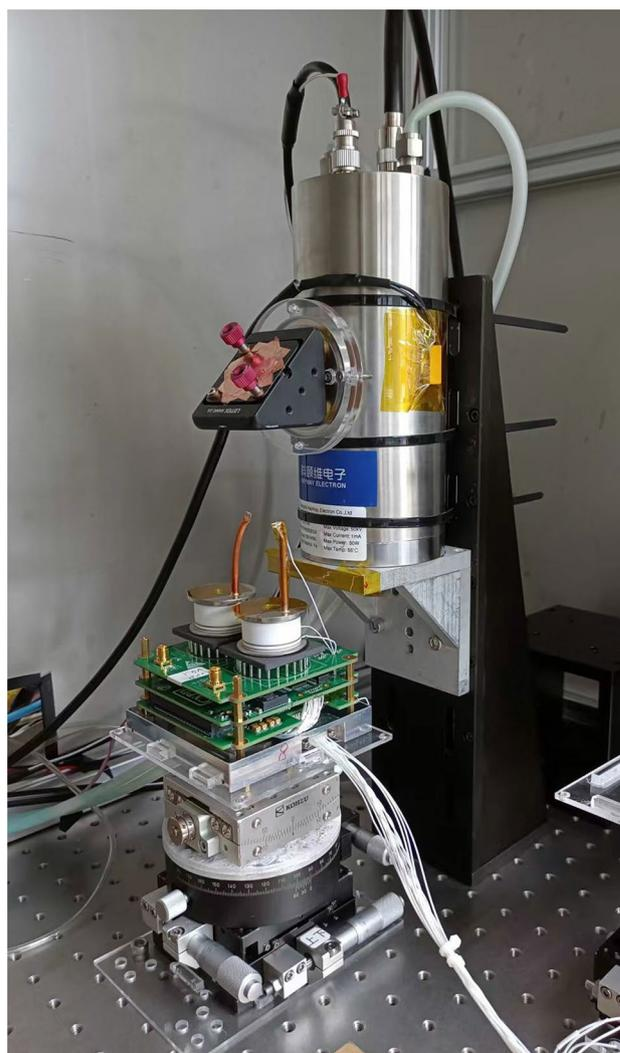
**Fig. 12** (Color online) The 8-mm height adapter pins were used for the test to replace the GPDs, and finally, both GPDs were directly soldered on the FEE board
